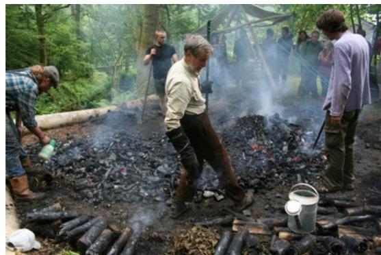
The mound was just over half of its starting size by the time we began to extinguish it. We poured water into it by means of a length of pipe thrust in to the sides. As the mud / turf cap was removed piece-by-piece we sprayed the remaining glowing areas with spray bottles to extinguish them. Our fears were unfounded — there were a few brown ends of course, but also a very respectable haul of charcoal. What a relief! All that remained was to rake it over, bag it up & tidy up the site.
